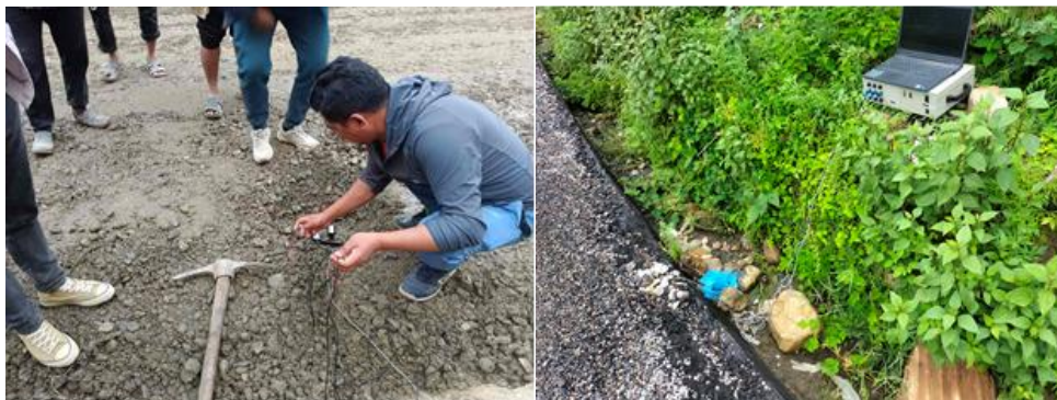
Figure 5. Field instrumentation and monitoring (strain gauge, earth pressure, and moisture): Use of sensors in unreinforced road section (Left Figure); Data monitoring setup (Right Figure)
